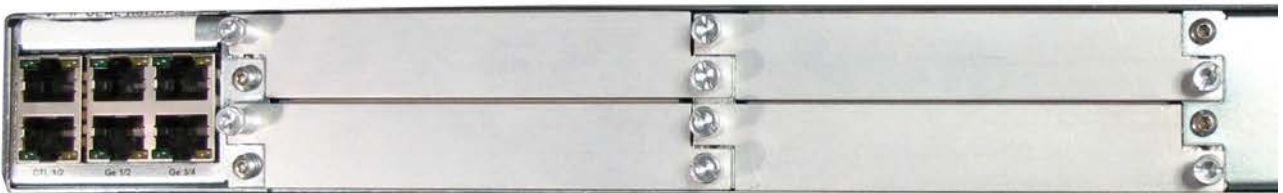
Rear View of the Ericsson SPR1100, dual DC PSU variant.
